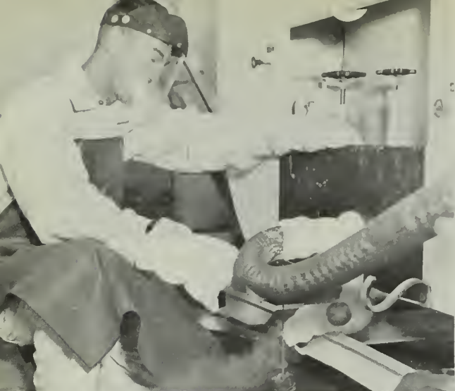
MACHINIST'S MATE fills stationary 500-gallon tank with liquid oxygen. Temperature of LOX is almost -300 degrees (note ice around coupling). Rt: Navyman prepares to purge LOX tank. Room where LOX is produced is in background.
